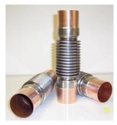
This range of small bore axial expansion joints are specifically designed to absorb the thermal expansion that occurs in hot water and perimeter heating circuits.
